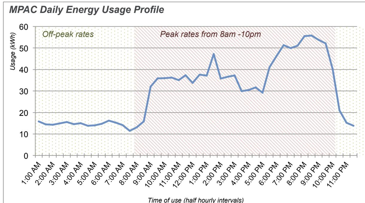
Through the Centre's Building Management System, MANPAC ensures that units are not left on when the Centre is not in use, loads are adjusted to suit conditions and the air conditioning is turned off in areas that are not in use. While the Centre's BMS is set up for timers, the usage of the MANPAC is not regular and staff has found it more expedient to adjust loads manually as required.
